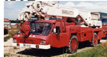
GB18 Haulotte, first «City crane» in the world - high travel speed, quick setting up and lifting cabin.
