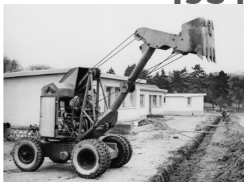
The SK2 compact shovel - the world's first tyre-mounted compact shovel with tailswing.
